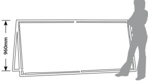
**2m footprint:** 2200 [w] x 650 [d]mm **3m footprint:** 3190 [w] x 650 [d]mm
